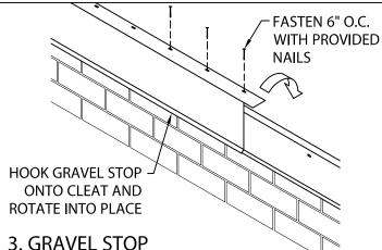
HOOK DRIP EDGE OF EACH GRAVEL STOP SECTION ONTO CONTINUOUS CLEAT, ROTATE INTO PLACE. FASTEN THRU PRE-SLOTTED HOLES 6" WITH PROVIDED NAILS.
