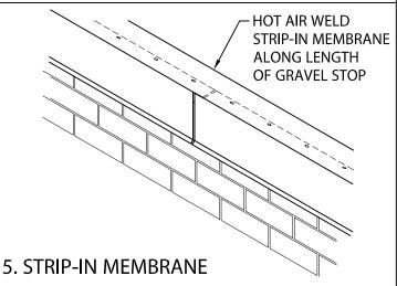
HOT AIR WELD STRIP-IN MEMBRANE ALONG ENTIRE LENGTH OF GRAVEL STOP PER MANUFACTURERS INSTRUCTIONS.
