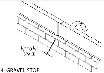
CONTINUE INSTALLING 12'-0" LENGTHS OF GRAVEL STOP. LEAVE A  $\frac{1}{8}$ " TO  $\frac{1}{4}$ " SPACE BETWEEN PIECES.
