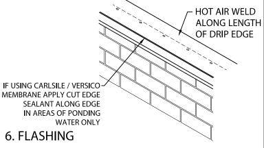
HOT AIR WELD ALONG ENTIRE LENGTH OF DRIP EDGE PER MANUFACTURERS INSTRUCTIONS. IF USING CARLSILE / VERSICO MEMBRANE, APPLY CUT EDGE SEALANT ONLY TO EDGES WHERE PONDING OCCURS.
