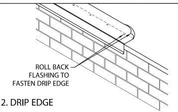
PLACE DRIP EDGE ON WALL. ROLL BACK FLASHING TO EXPOSE FASTENING SLOTS AND FASTEN THRU PRE-SLOTTED HOLES 6" WITH PROVIDED NAILS.
