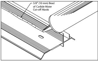
2. Miter & Scupper Anchor Bar (Preparation) Lay miters and spillout scuppers on deck with outside face down. Be sure aluminum anchor bar is clean and free of dirt or dust. Apply a heavy 3/8" (10 mm) bead of Carlisle Water Cut-Off Mastic to the right angle intersection of the deck flange and back of anchor bar as shown. Application of sealant is required along the full length of each miter anchor bar.
