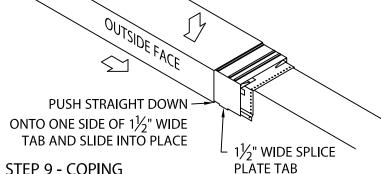
PUSH COPING STRAIGHT DOWN INTO PLACE ONTO ONE SIDE OF 1½" WIDE SPLICE PLATE TAB. CONTINUE DOWNWARD PRESSURE UNTIL SNAP LOCK OCCURS ON BOTH LEGS. SLIDE COPING OVER TAB SO THAT HALF OF SPLICE PLATE IS SHOWING.
