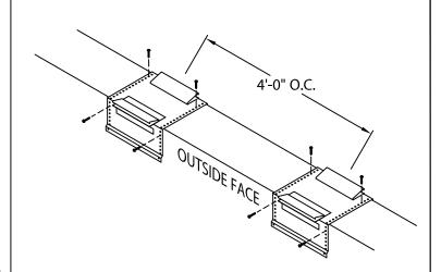
STEP 7 - ANCHOR CLIPS LOCATE AND FASTEN GALVANIZED ANCHOR CLIPS TO WALL AT 4'-0" CENTERS WITH PROVIDED FASTENERS FOR SUBSTRATE (SEE DETAIL A).
