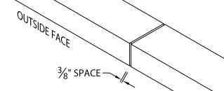
STEP 10 - COMPLETION CONTINUE INSTALLING COPING WITH A 3/8"
