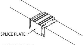
**STEP 8 - SPLICE PLATES** PLACE SPLICE PLATE ONTO ANCHOR CLIPS AT SPLICE JOINTS, 12'-0" O.C. NOTE: REMOVE RELEASE PAPER FROM SEALANT STRIPS.
