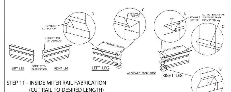
RIGHT LEG - DETAIL A: FIRST REMOVE SECTION 1/8" DOWN AND 1" HORIZONTALLY AS SHOWN TO CREATE TAB. TRIM TOP FLANGE BACK AT A 45° ANGLE. DETAIL B: CUT OFF BOTTOM FACE 1/8" AS SHOWN AND CONTINUE CUT AT A 45° ANGLE THROUGH AREA SHOWN ON BOTTOM FLANGE. DETAIL C: CUT OUT BIRD'S CUT BOTTOM BEAK STIFFENING BAND FROM 1" TAB. BEND TAB INWARDS 90°.
