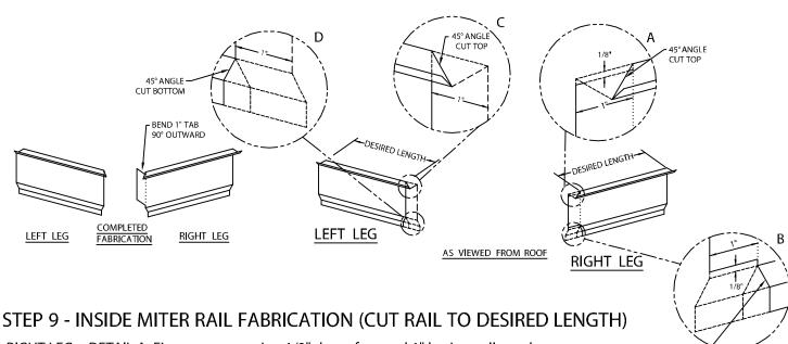
RIGHT LEG - DETAIL A: First remove section 1/8" down face and 1" horizontally as shown to create tab. Trim top flange back at a 45° angle. DETAIL B: Cut off bottom face 1/8" as shown and continue cut at a 45° through area shown on bottom flange. Bend tab inwards 90°. LEFT LEG - DETAIL C: Cut top flange at a 45° angle. Continue down face. DETAIL D: Cut bottom flange at 45° angle as shown.
