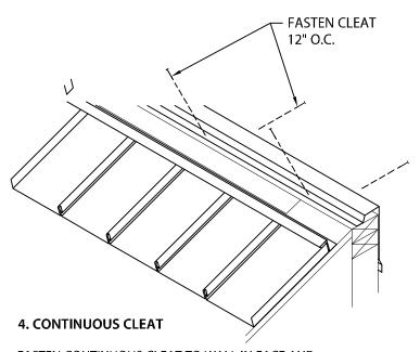
FASTEN CONTINUOUS CLEAT TO WALL IN FACE AND TOP FLANGE 12" O.C. AS SHOWN USING APPROPRIATE FASTENERS FOR SUBSTRATE.
