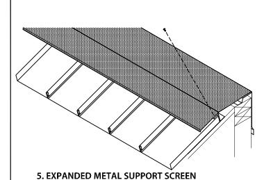
PLACE SCREEN CENTERED OVER "Z" BRACKETS. TEMPORARILY FASTEN TO "Z" BRACKETS AT EACH END OF 12'-0" LENGTH TO HOLD IN PLACE.
