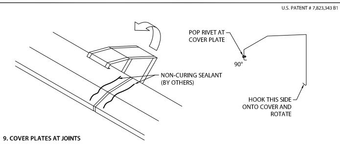
APPLY A GENEROUS BEAD OF NON-CURING SEALANT (BY OTHERS) TO EACH SIDE OF JOINT. HOOK COVER PLATE ONTO COVER AT JOINTS AND ROTATE INTO PLACE. POP RIVET INTO COVER PLATE AT ONE SIDE OF THE JOINT (FASTEN SIDE WHICH HAS 90° DRIP ANGLE). THIS WILL PREVENT MIGRATION.
