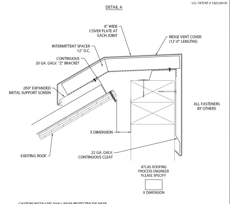
CAUTION! INSTALLERS SHALL WEAR PROTECTIVE EYE WEAR TO PREVENT INJURY. DO NOT OVERDRIVE FASTENERS, AS STRIPPING CAN OCCUR AT HIGH DRIVER TORQUE. RECOMMENDED DRIVING TOOL: 600 - 800 rpm ELECTRIC DRILL EQUIPPED WITH DEPTH-SENSING NOSE-PIECE TO PREVENT DRIVING AND STRIPOUT. DO NOT USE IMPACT TYPE TOOL.
