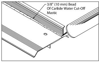
2. Miter & Scupper Anchor Bar (Preparation) Lay miters and spillout scuppers on deck with outside face down. Be sure aluminum anchor bar is clean and free of dirt or dust. Apply a heavy 3/8" bead of Carlisle Water Cut-Off Mastic to the right angle intersection of the deck flange and back of anchor bar as shown. Application of sealant is required along the full length of each miter anchor bar.
