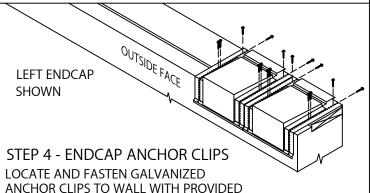
FASTENERS FOR SUBSTRATE (SEE DETAIL A).
