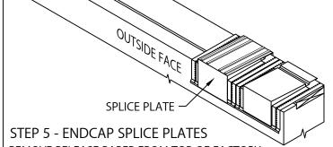
REMOVE RELEASE PAPER FROM TOP OF FACTORY APPLIED DUAL NON-CURING SEALANT STRIPS. PLACE SPLICE PLATE ONTO SECOND ANCHOR CLIP AS SHOWN.
