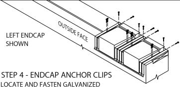
LOCATE AND FASTEN GALVANIZED ANCHOR CLIPS TO WALL WITH PROVIDED FASTENERS FOR SUBSTRATE (SEE DETAIL A).
