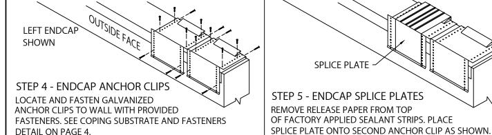
SPLICE PLATE STEP 5 - ENDCAP SPLICE PLATES REMOVE RELEASE PAPER FROM TOP OF FACTORY APPLIED SEALANT STRIPS. PLACE
