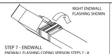
HOOK OUTSIDE FACE OF ENDWALL OVER THE ANCHOR CLIPS AND ROTATE INTO PLACE. ENGAGE REAR LEG ONTO ANCHOR CLIPS BY PRESSING DOWNWARD UNTIL
