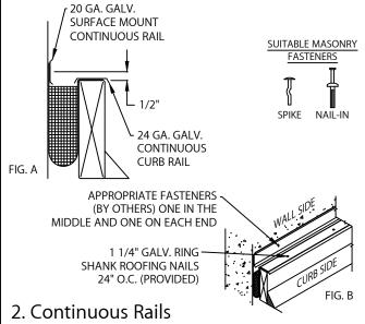
Fasten the 24 ga. galvanized continuous curb rail 24" O.C. to the top of the wood curb with provided 1 1/4" galvanized ring shank roofing nails (Fig. B). Fasten the 20 ga. galvanized surface mount continuous rail (edges facing out) to the wall (one fastener in the middle and one at each end) with an appropriate fastener (by others) suitable for substrate, with flatest head possible (see above). The center of the surface mount rail must be 1/2" above the top of the wood curb (Fig. A)
