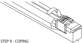
HOOK OUTSIDE FACE OF COPING OVER THE ANCHOR CLIPS AND ROTATE INTO PLACE. ENGAGE REAR LEG ONTO ANCHOR CLIPS BY PRESSING DOWNWARD UNTIL SNAP LOCK OCCURS.
