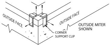
STEP 1 - CORNER SUPPORT CLIPS LOCATE AND FASTEN GALVANIZED CORNER SUPPORT CLIPS TO THE WALL.
