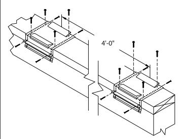
STEP 7 - ANCHOR CLIPS LOCATE AND FASTEN GALVANIZED ANCHOR CLIPS TO WALL AT 4'-0" CENTERS WITH PROVIDED FASTENERS FOR SUBSTRATE (SEE DETAIL A).
