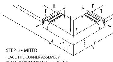
INTO POSITION AND SECURE AT THE EXPOSED EDGE OF THE ANCHOR CLIPS AS PER DETAIL A.
