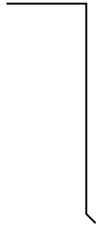
24 GA. GALV. CONTINUOUS BACKER CLEAT, 12'-0" LENGTHS
