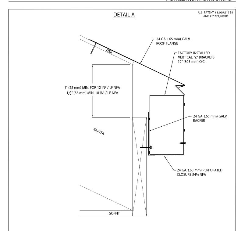
SUBSTRATE MUST BE CONTINUOUS, FLAT, VERTICAL, AND ABLE TO SUPPORT FASTENERS WITH A MINIMUM 240 LB. PULL-OUT.
