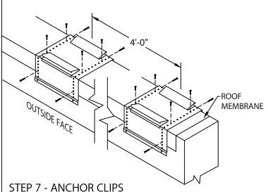
LOCATE OVER ROOFING MEMBRANE
