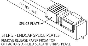
SPLICE PLATE ONTO SECOND ANCHOR CLIP AS SHOWN.
