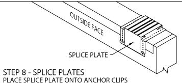
NOTE: REMOVE RELEASE PAPER FROM SEALANT STRIPS.
