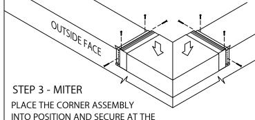
EXPOSED EDGE OF THE ANCHOR CLIPS AS PER DETAIL A.
