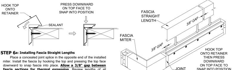
downward to snap fascia into place. Allow a 3/8" gap between fascia sections for thermal expansion. Review lengths of all straight pieces prior to cutting to avoid creating relatively short sections of fascia adjacent to full length sections. (DO NOT HOOK THE BOTTOM OF THE SPLICE ONTO THE RETAINER) Note: There must be a splice at every joint.
