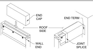
(DO NOT HOOK THE BOTTOM OF THE SPLICE ONTO THE RETAINER)
